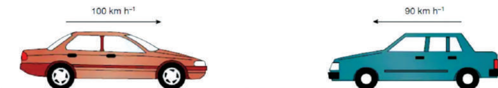
(b) The velocity of the car approaching from the left relative to the observer is 190 \text{ km h}^{-1} due east.
